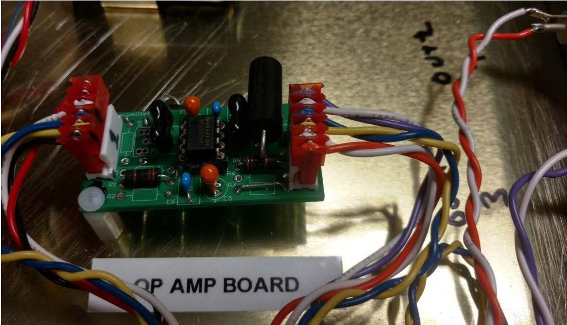
Figure 19 Op amp board configured for circuit evaluation with wirewound resistors
