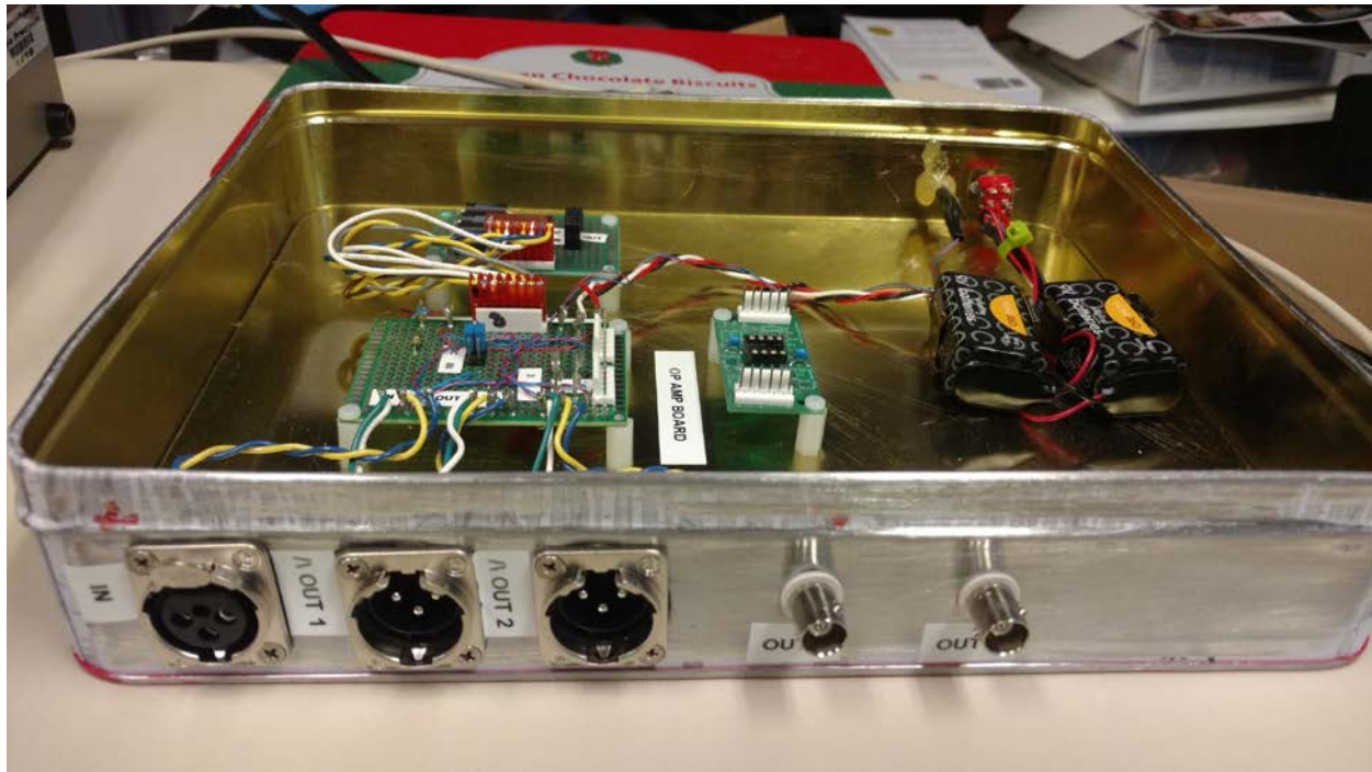
Figure 17 System construction (rear panel, prior to op amp board connection)
