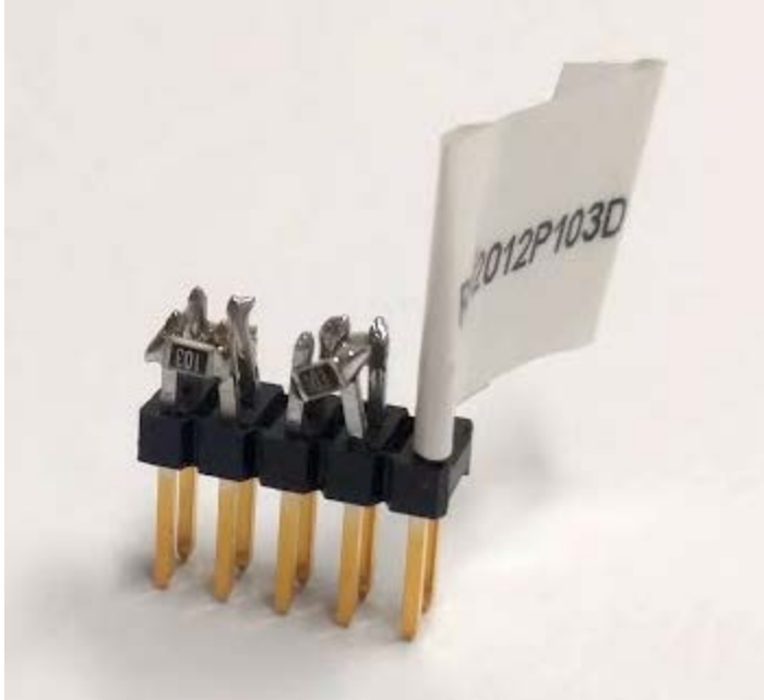
Figure 25 Unshrouded header for resistors. A little fragile but is easier to mate correctly than the shrouded one
