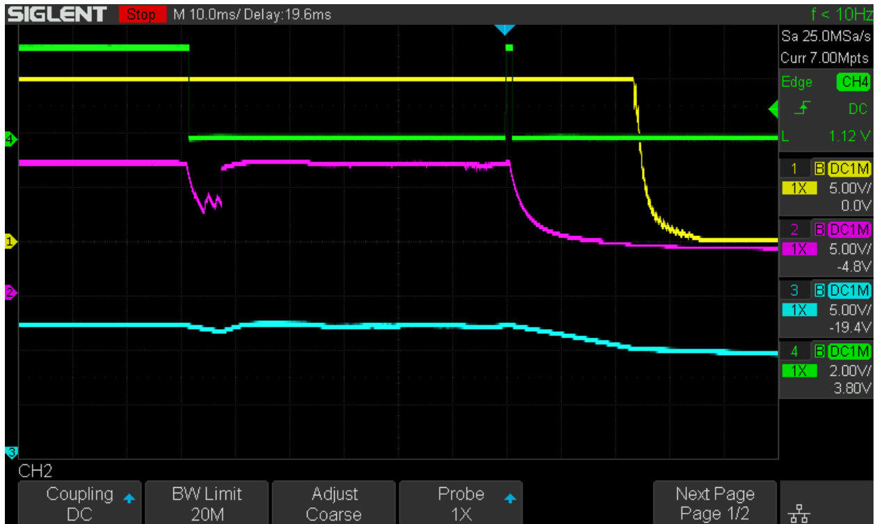
Figure 9 Small PowerGood pulse caused by just the right timing of events. +15V (ch1) Yellow, 12V input (ch2) Magenta, 12V local (ch3) Blue, PowerGood (ch4) Green
