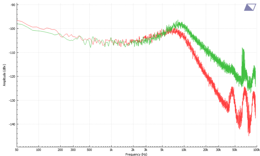
Figure 6 LTC7151 without extra filter (Green) and with filter (Red)
