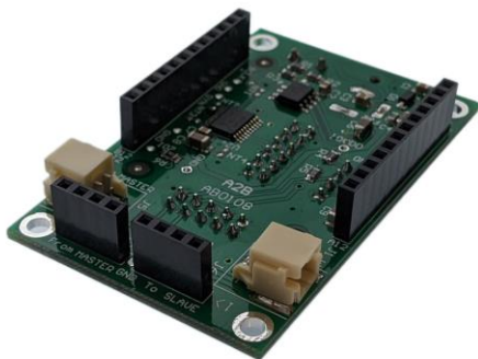
Figure 4 AB0108 root node, external clock, I/O expander (mates with OEM A 2 B module)
