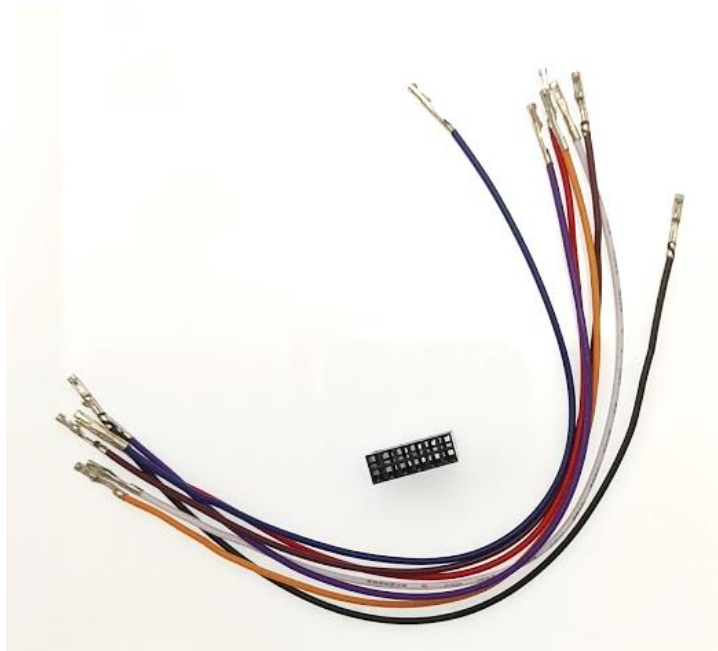
Figure 19 Typical .1" shell and precrimped wires (these are crimped both ends)
