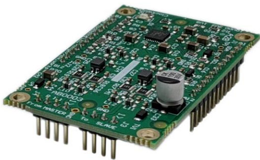
Figure 3 OEM A2B module – locally powered version (AB0003L)
