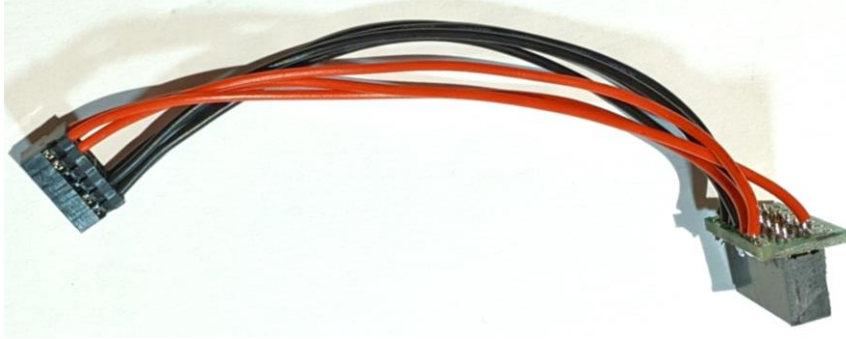
Figure 5 I 2 S cable example to connect MCHStreamer board to AB0108
