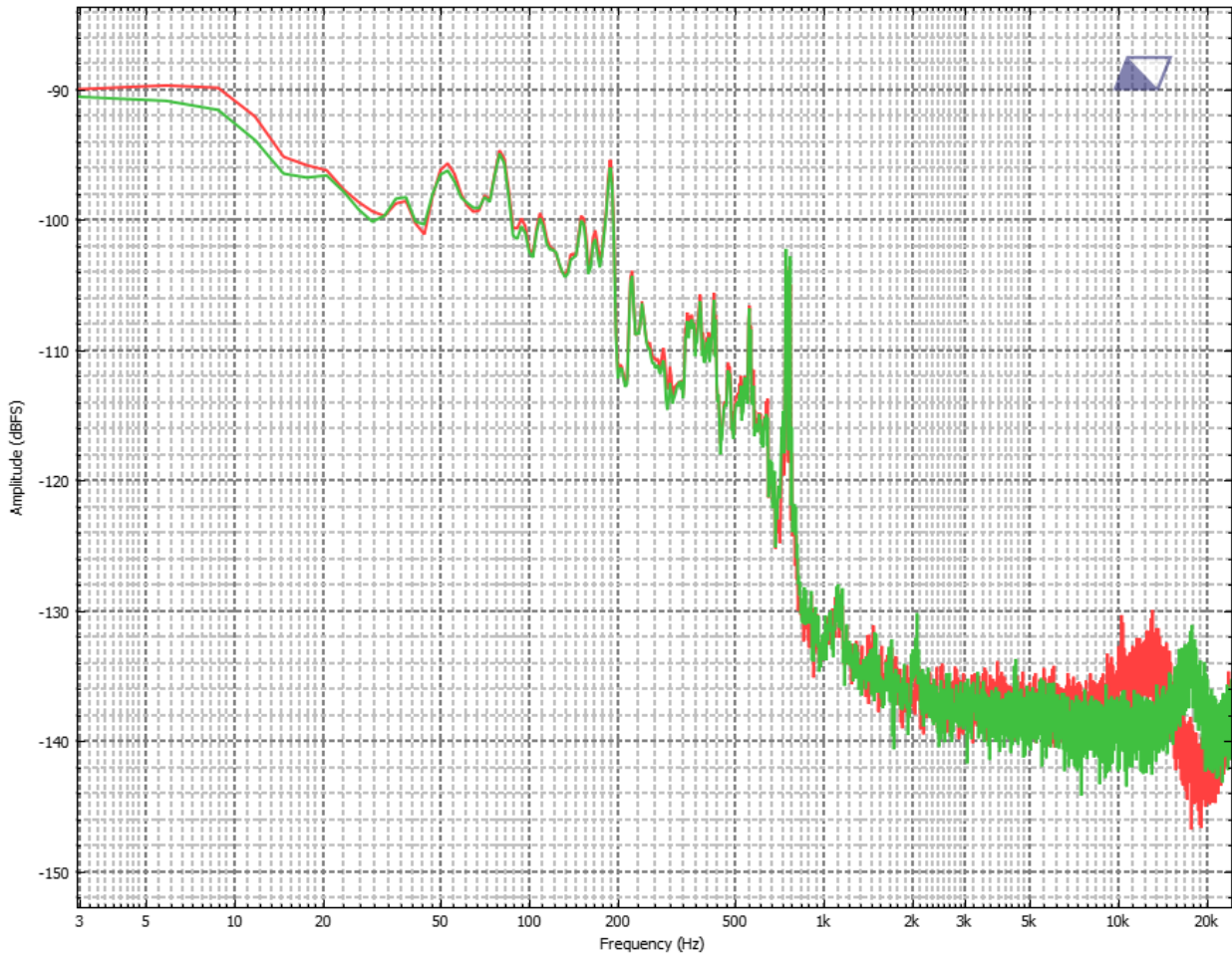
Typical noise floor from two of the four microphones when acoustically semi-isolated. 16K point FFT, 16 averages. Approx -85 dBFS RMS signal level.
