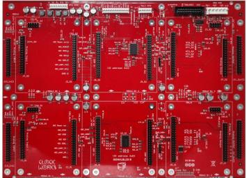
Input and output follows the SignalBlox convention with a 40 pin connector providing 8 balanced analog I/O per section; the CC0003's two sections therefor provide 16 in and 16 out capability.
