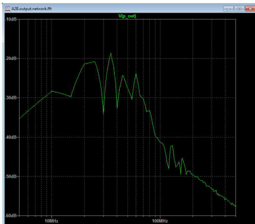
Figure 12 Output spectrum using a short simulated length of Manchester encoded data. A more detailed/longer run would be needed to get an overall smooth spectrum.
