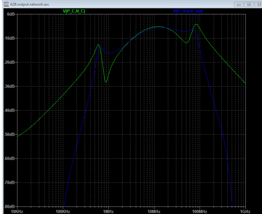
Figure 11 Frequency response plots at same places as waveforms in Figure 10
