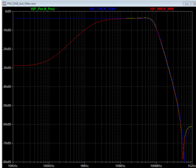
Figure 4 Comparison of the 3 models. Green with simple inductor, Blue with the precision TDK model, and simple models with the extra filter section.
