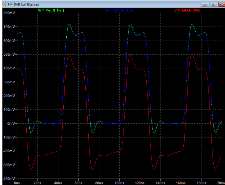
Figure 6 Time domain view of pulse waveform similar to A 2 B data.
