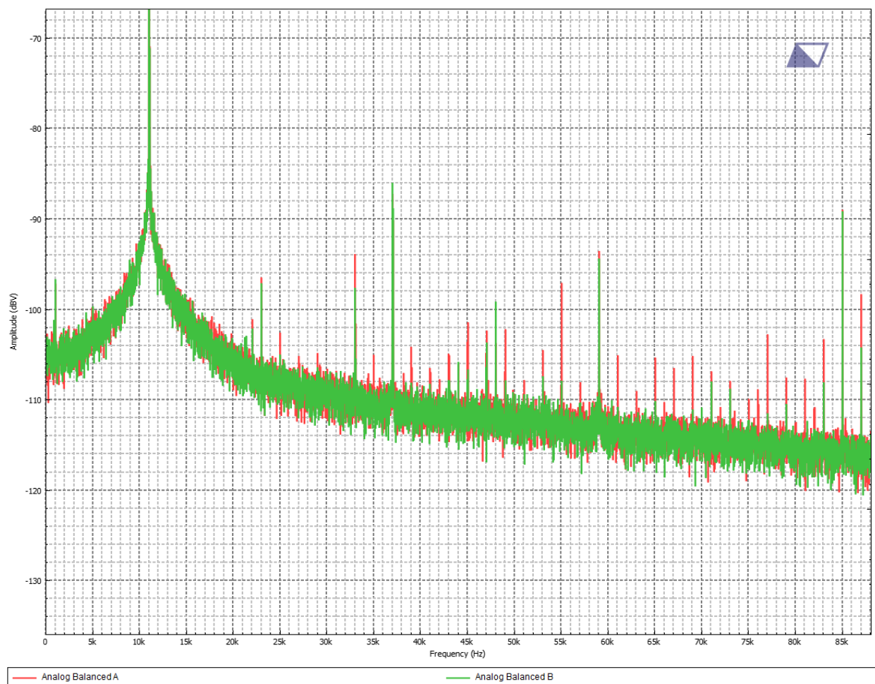
Figure 18 Node 4 11 kHz -1 dBFS output - wide band view (32K pt FFT)
