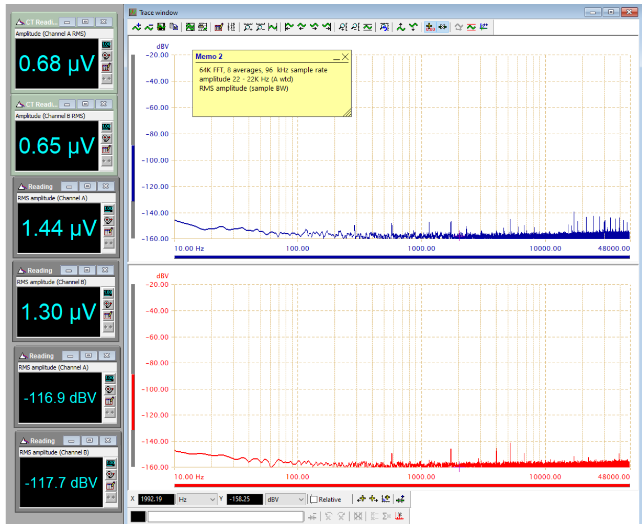
Figure 28 dScope M1 with input shorted, measured 7-Apr-23
