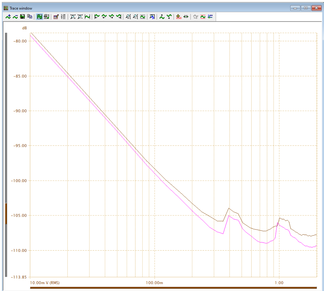
Figure 8 THD+N vs. level to show effect of auto ranging, Brown = Chan A, Purple = Chan B
