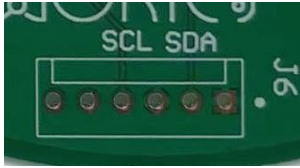
Figure 15 External/Aux control connector
