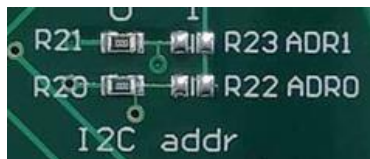
Figure 11 LPC5024 base address jumpers
