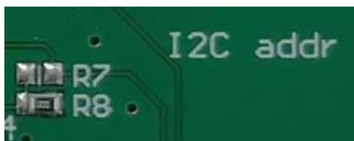
Figure 9 ADAU7118 base address jumper
