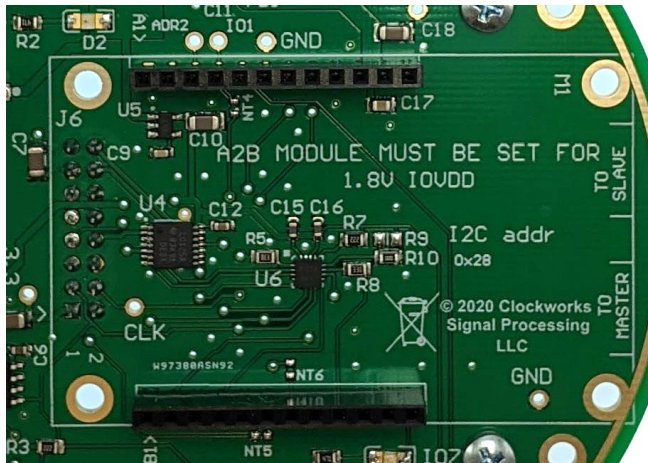
Figure 12 A 2 B module connector location on PDM to I 2 S board
