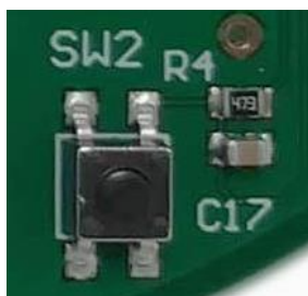
Figure 7 User switch location on PDM to I2S board
