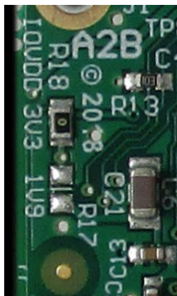
Figure 16 Rev 2: IOVdd jumper resistors. 3.3V is the factory default
