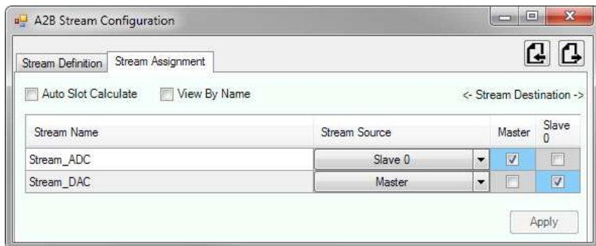
Figure 32 Simple stereo stream routing for two EVM example
