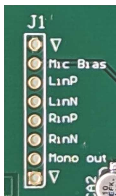
Figure 6 ADAU1761 microphone input signal breakout
