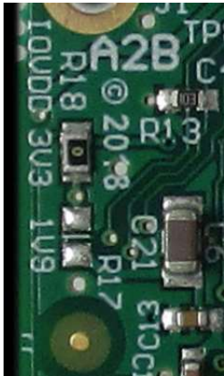
Figure 14 Rev 2: IOVdd jumper resistors. 3.3V is the factory default
