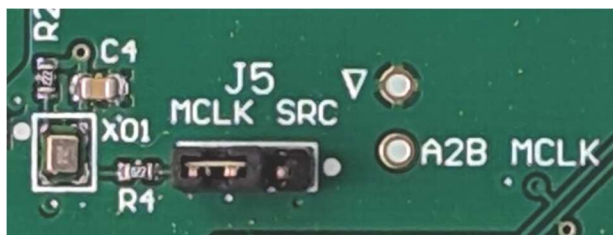
Figure 7 MCLK jumper for local oscillator
