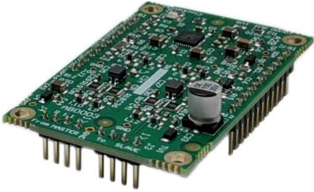
Figure 3 OEM A²B module - locally powered version (AB0003L)
