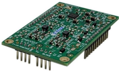
Figure 4 OEM A²B module - phantom powered version (AB0003P)
