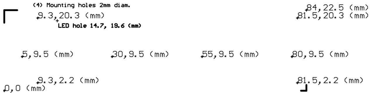
Figure 2 AB0204 dimensions and hole locations
